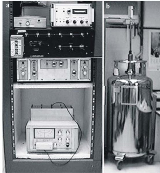
Figure 2.1- Overview of the CCC based resistance bridge. a) Bridge electronics (from top to bottom): integrator, SQUID readout, “difference compensator”, current sources, two test 100 \Omega resistors (inside an Al box) and nano-voltmeter; b) transportable Dewar with telescopic insert.
